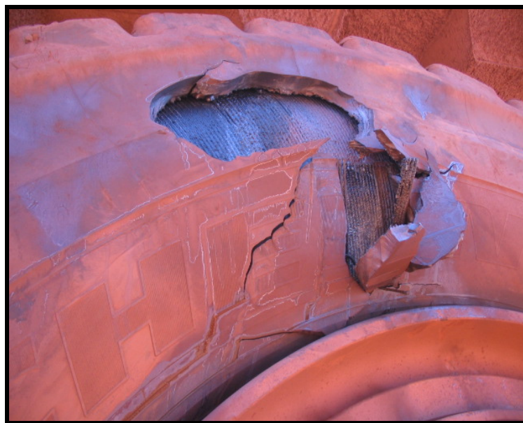
Figure 2: Sidewall of position 3 tyre where burst occurred
