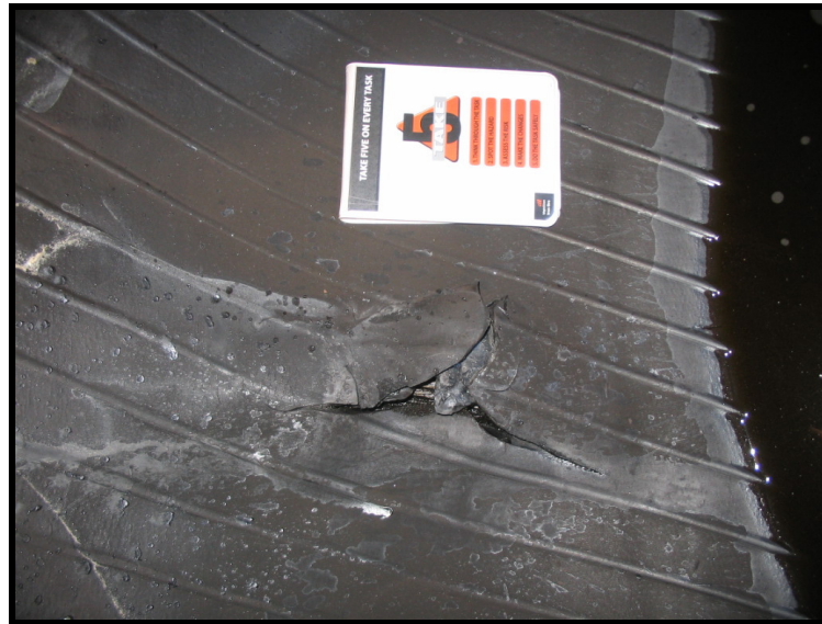
Figure 1: Split in the inner liner of position 3 tyre
