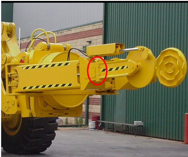
Figure 1 – Example of a “bolt on” component
