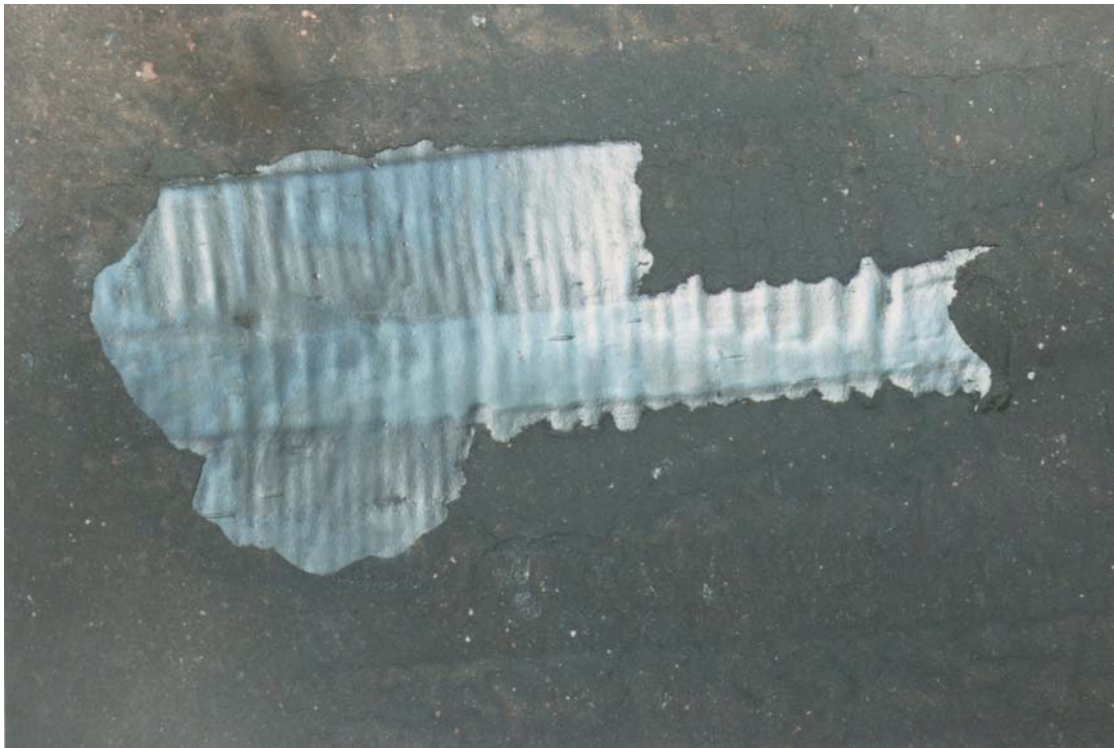
Figure 4 - Internal of tyre showing pyrolyzed area and arcing point.
