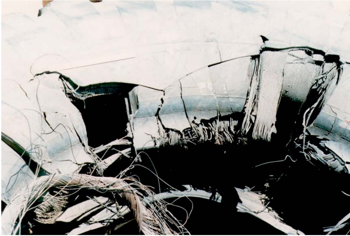
Figure 3 - The Damaged Bead Area
